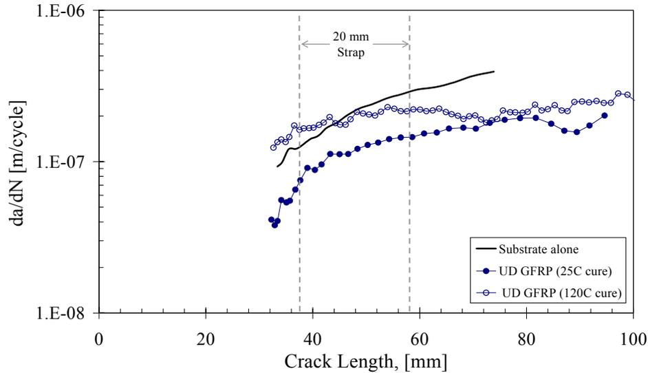
Figure 5 Crack growth rate plotted against crack length for grp strap;  $\mu=0.016$ , showing influence of residual stress
