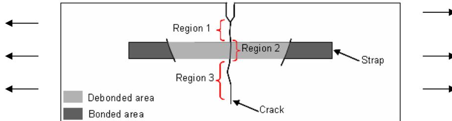
Figure 2 Illustration of the regions of influence of a bonded strap on a crack propagating in a substrate
