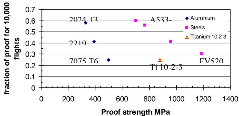
Figure 1 The influence of static strength and alloy type on the largest peak stress in the TWIST spectrum at which 10,000 flights can be achieved. The stress is expressed as a fraction of the proof strength of the alloy.
