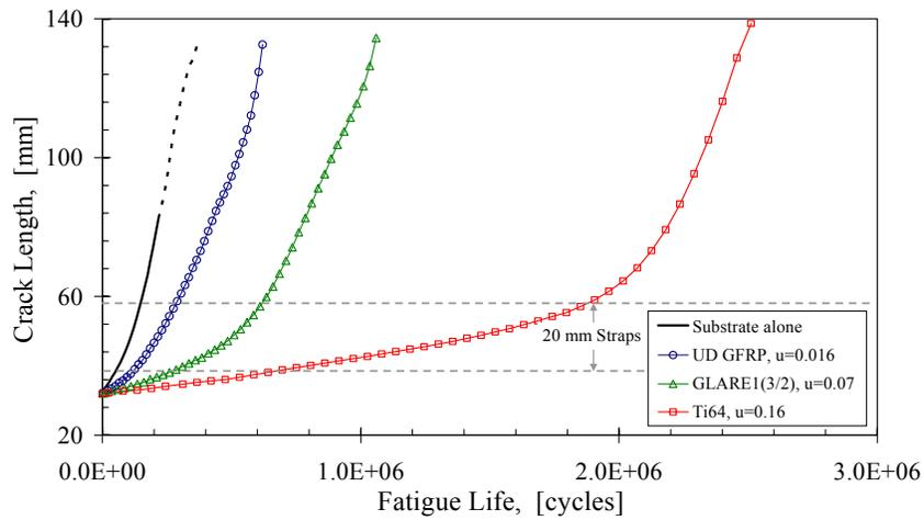
Figure 4 Crack length vs. cycles for the test data shown in figure 3, showing the effect of  $\mu$  value on the total lives to failure
