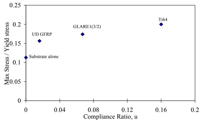
Figure 6 Increases in applied stress to achieve a crack growth life of  $10^5$  cycles with increasing  $\mu$  value, expressed as a fraction of yield strength. Room temperature cure adhesive.
