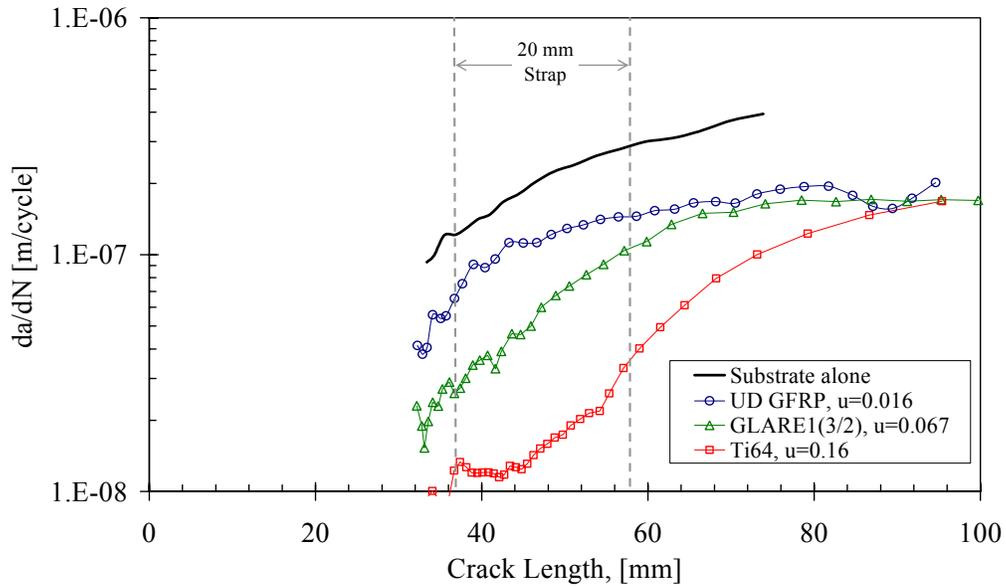
Figure 3 Fatigue crack growth rates plotted against crack length for different strap materials with different  $\mu$  values. The behaviour of the substrate alone is also shown. All samples with room temperature cure
