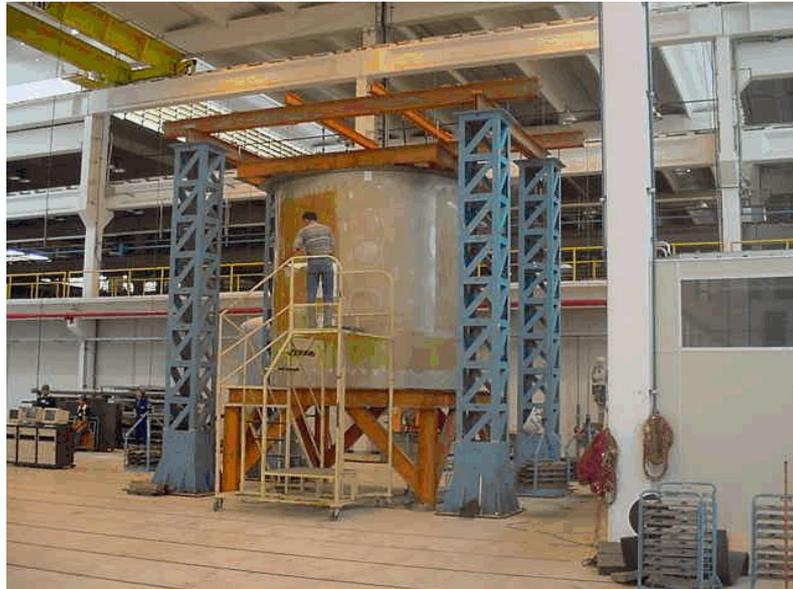
Figure 3: Overview of 170 fuselage barrel fatigue test specimen
