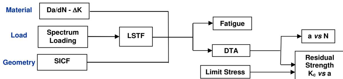
Figure 2: Overview of fatigue and DT analysis procedure
