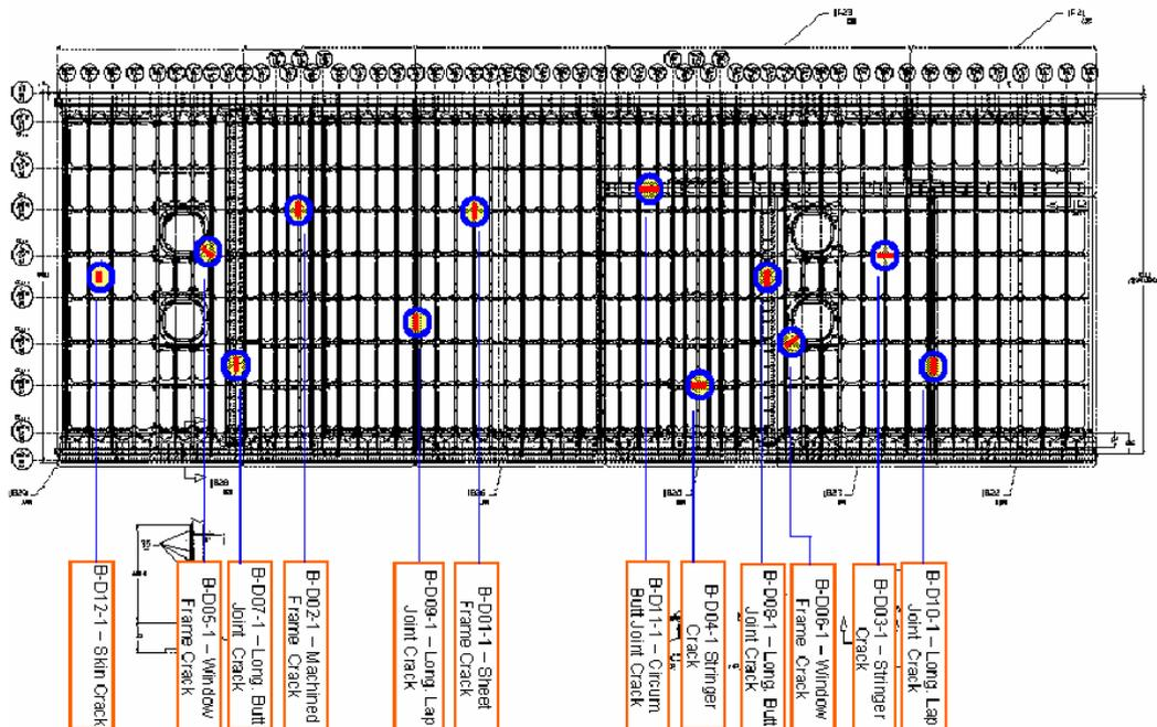
Figure 4 – Outline of induced damages for Phase I
