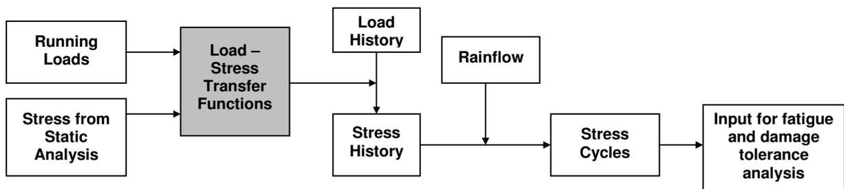
Figure 1: Overview of fatigue and DT analysis procedure
