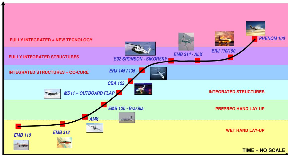
Figure 5 – Evolution of composite applications in Embraer aircraft
