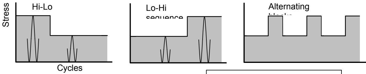
Fig.7a: Simple block loading.
