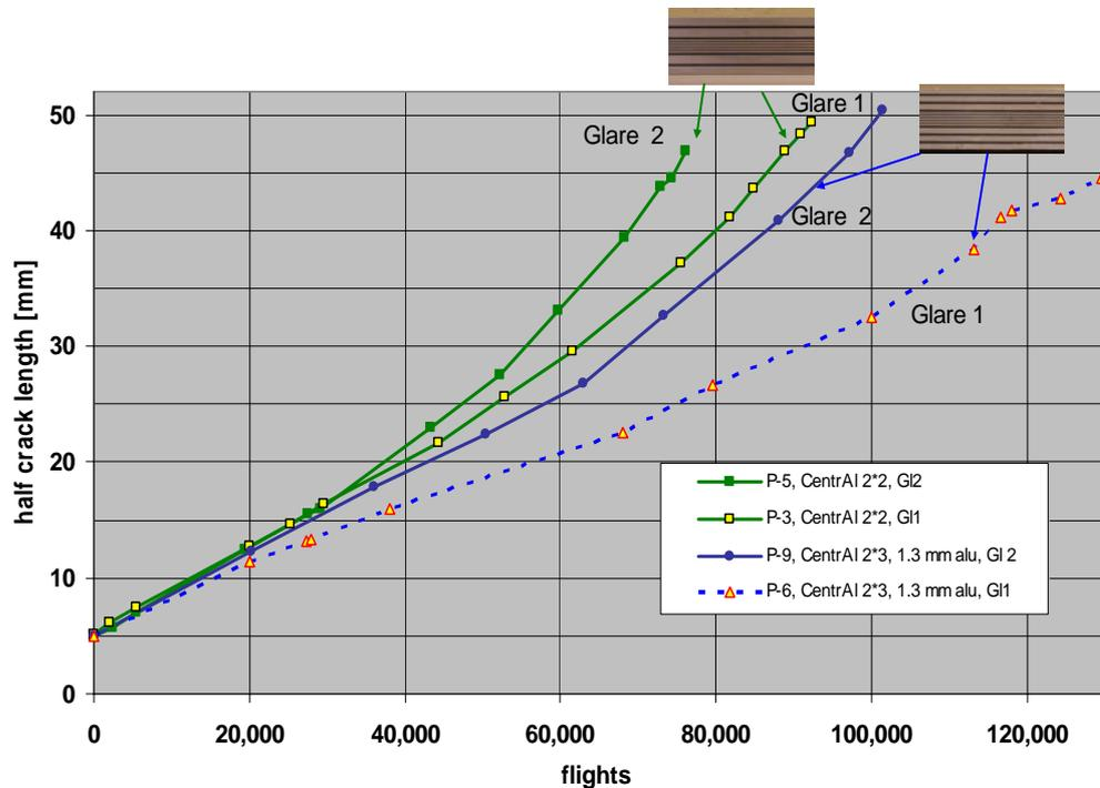
Figure 11: The influence of the Glare type used in CentrAl on fatigue crack growth under mini-TWIST fatigue loading.
