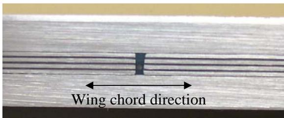
Figure 16: Butt-splice in Glare layer
