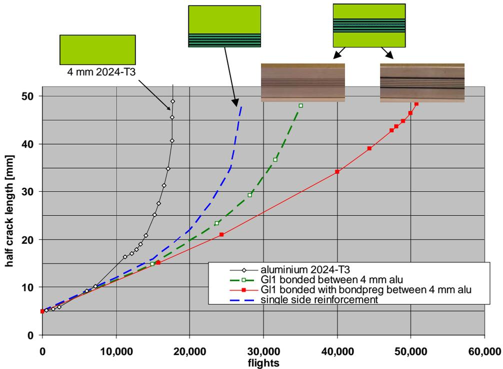
Figure 8: Fatigue crack growth behaviour for center cracked specimen under mini-TWIST fatigue loading (Smsf = 100 MPa, GTA = -0.1, trunc. = 1.15)
