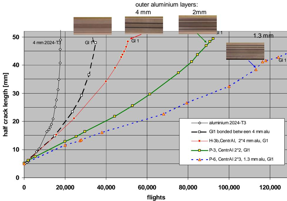
Figure 10: The effect of the thickness of the outer aluminium layers on fatigue crack growth in CentrAl (mini-TWIST loading)
