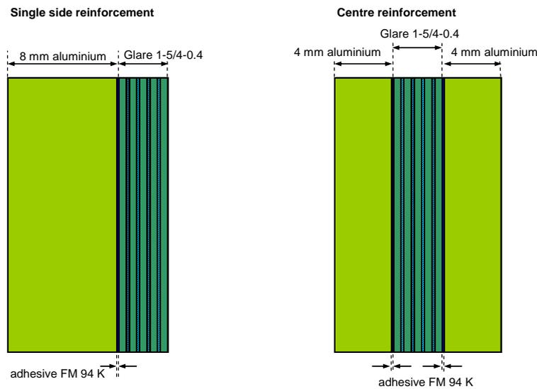
Figure 3: Cross sections of single side and centre reinforced aluminium
