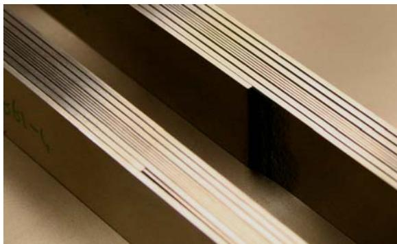
Figure 17: Ply drop off in CentrAl
