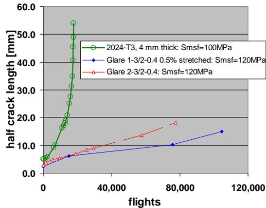
Figure 1: Fatigue crack growth in aluminium and Glare under spectrum loading
