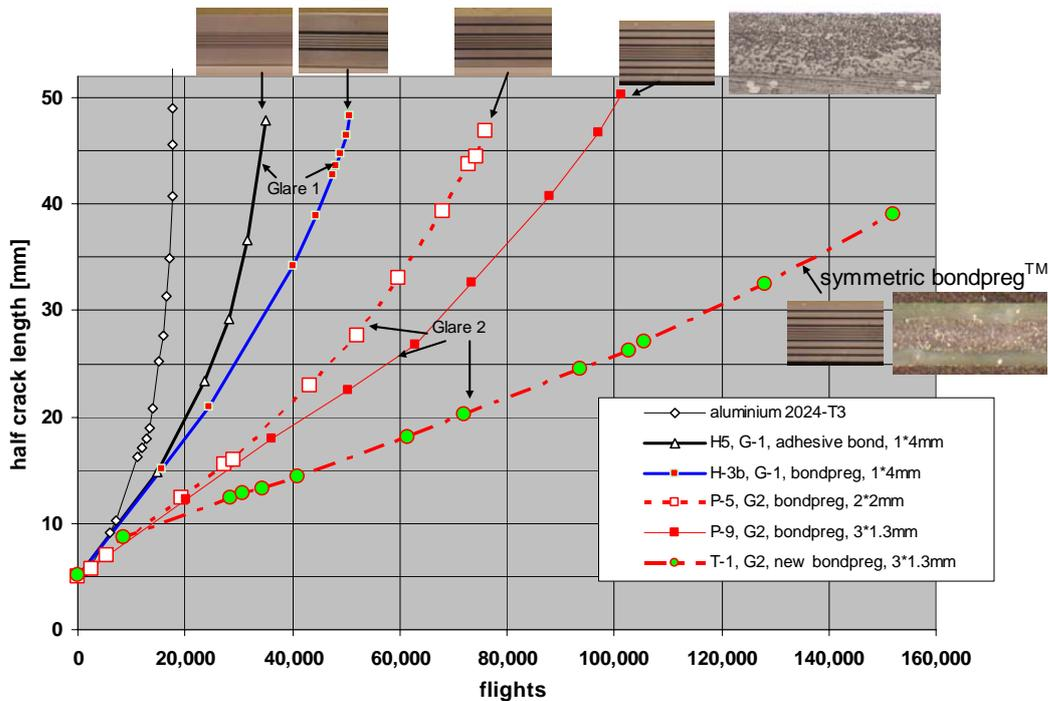
Figure 13: Reduced crack growth rates in CentrAl with symmetric bondpreg™
