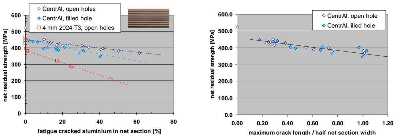
Figure 14: Residual net strength of fatigued blunt notch specimen
