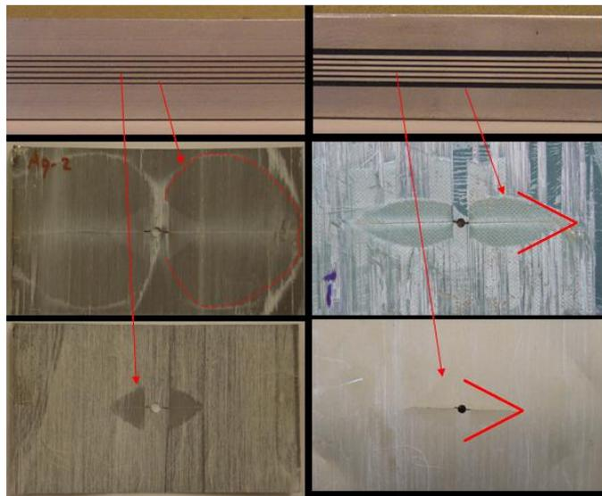
Figure 7: Comparison of delamination areas for adhesive (left) and bondpreg<sup>TM</sup> based materials.
