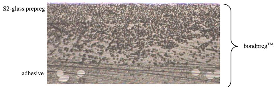
Figure 6: Bondpreg<sup>TM</sup> cross section
