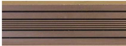
1970: Lockheed Tristar: Titanium straps bonded on (thin) aluminium skin improves the structures residual strength.
