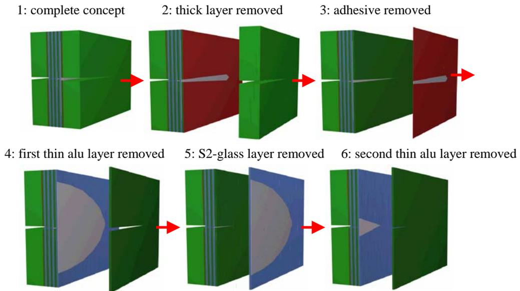
Figure 4: Fatigue cracked material concept, layers removed step by step
