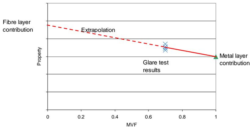
Figure 15: The Metal Volume Fraction approach
