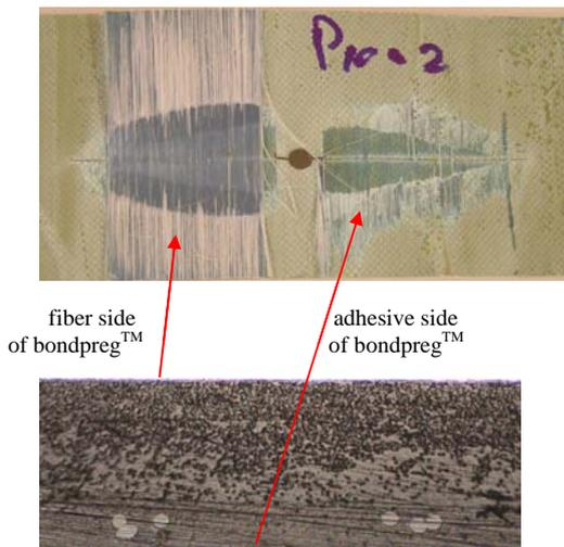
Figure 12: Unequal delamination size at both interfaces of non-symmetric bondpreg
