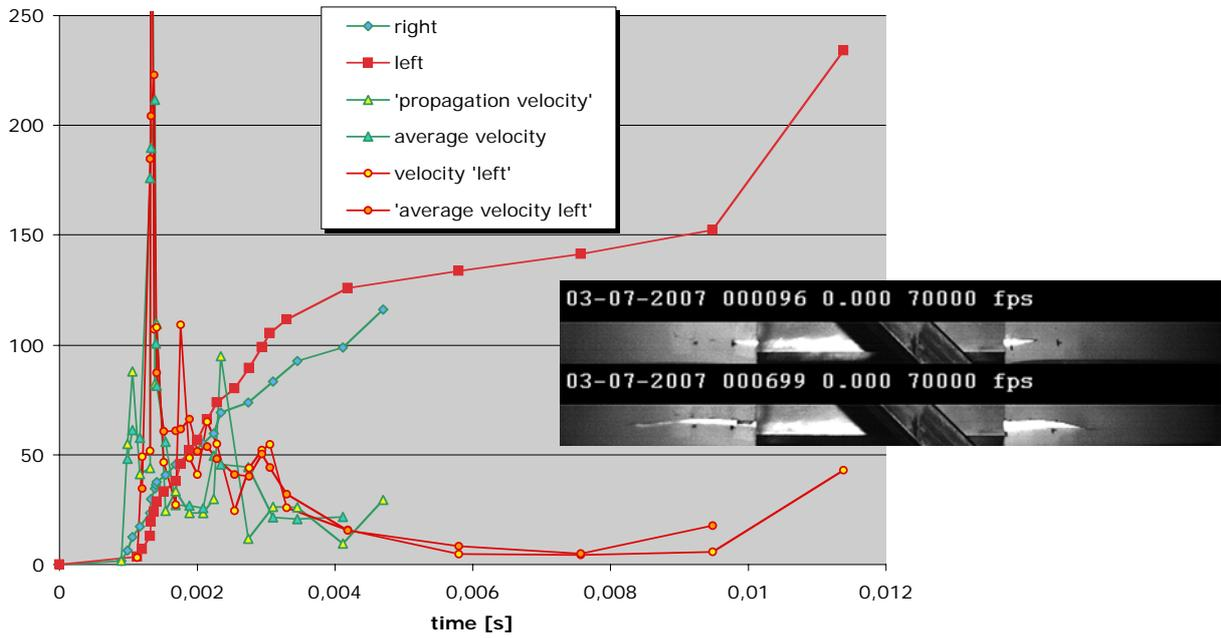
Figure 6: Crack propagation velocity for experiment 4 with initial crack 280 mm and 260 mm crack extension path on both ends.
