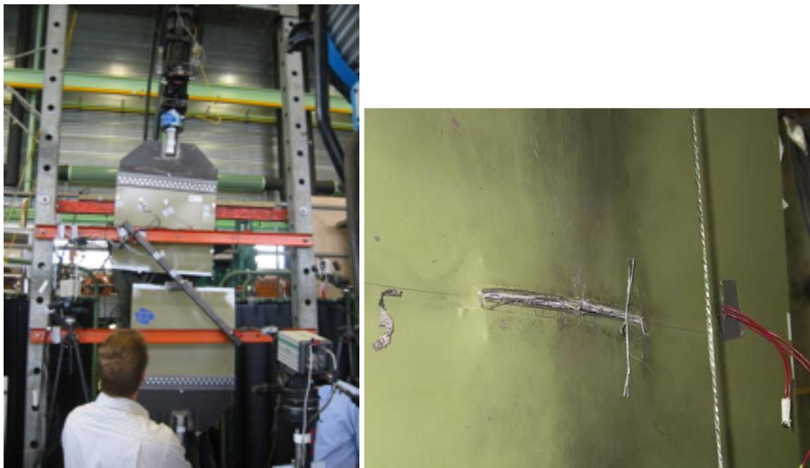
Figure 4: Test set-up uniaxial ECCT test with sudden crack initiation after failure in test 2 (left) and a close-up of the 200 mm 'sudden crack' as generated in test 1 (right); note the appearance of broken fibers.
