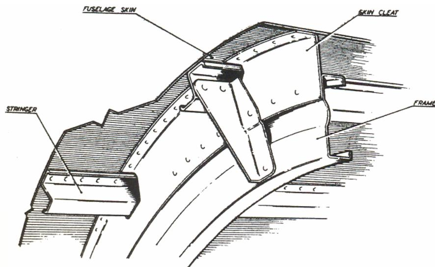
Figure 1: Example of a critical design feature: the frame-skin joint or castellation (VC10/BAC-111)
