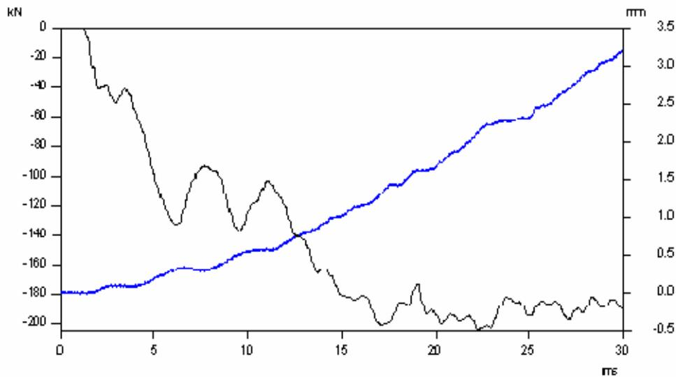
Figure 8: Displacement (blue) and force (black) of hydraulic jack after the explosive cut initiation.
