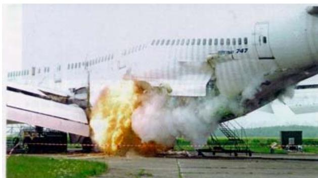
Figure 2: Catastrophic failure behaviour demonstrated in the 2001 DERA test
