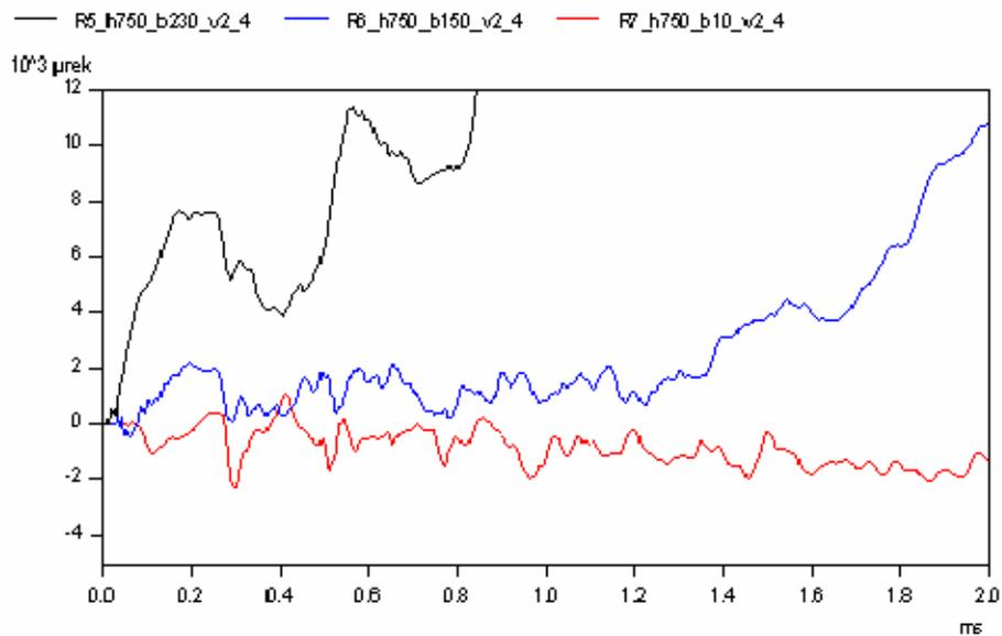
Figure 9: Strain change next to the crack during the first two milliseconds after cut initiation (strain gauge positions as in Figure 7).
