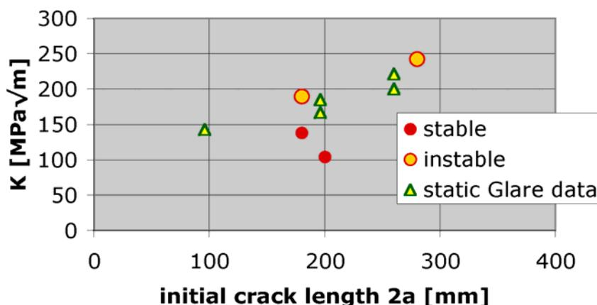
Figure 5: Crack stability plot of current experiments compared to literature data (based on initial crack length)
