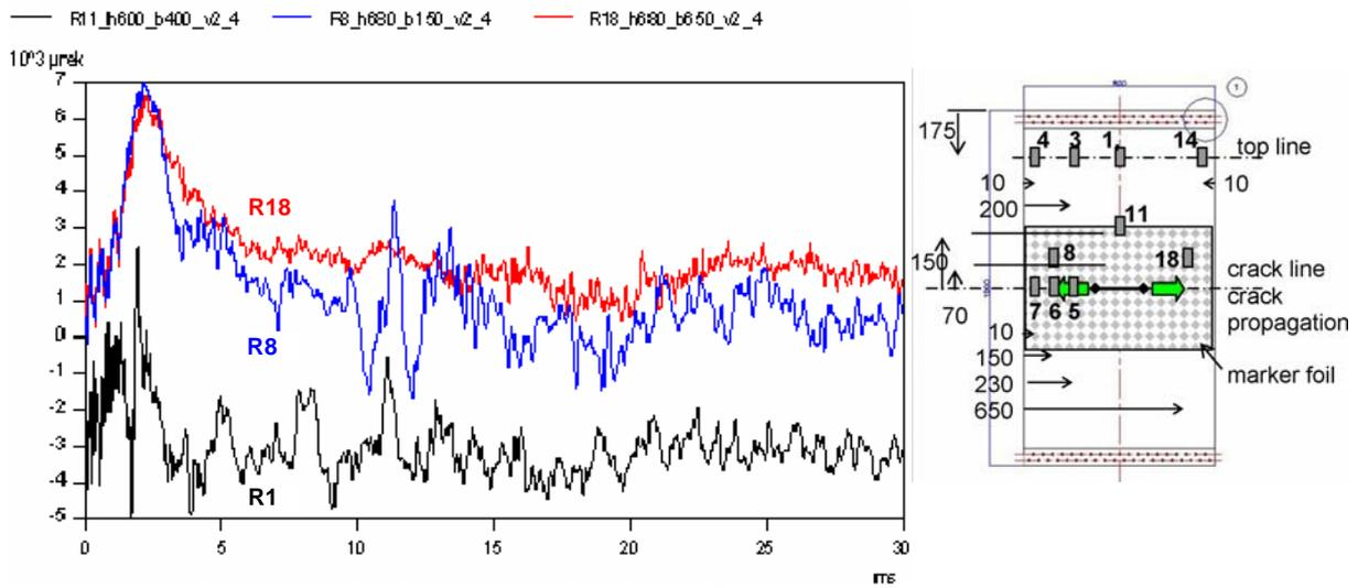
Figure 7: Strain change versus time (in ms) for central and side gauges (#11, 8, 18)
