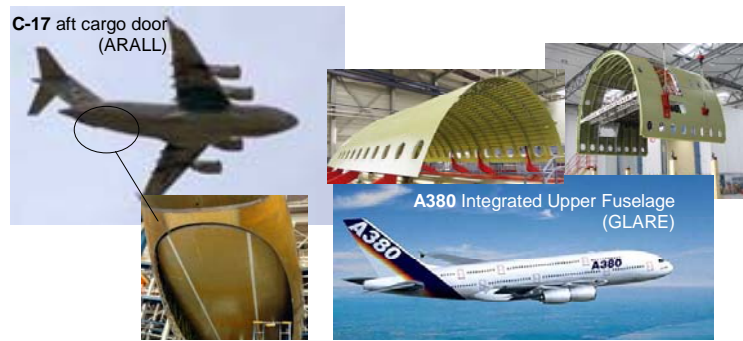
Figure 2. Applications of FML structures on C-17 and A380 aircraft
