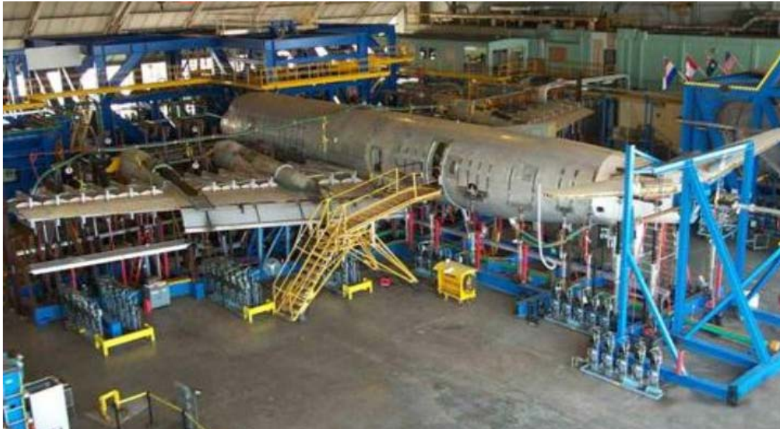
Figure 1: P-3 SLAP Wing/Fuselage Fatigue Test Article and Rig at Lockheed-Martin, Marietta, GA
