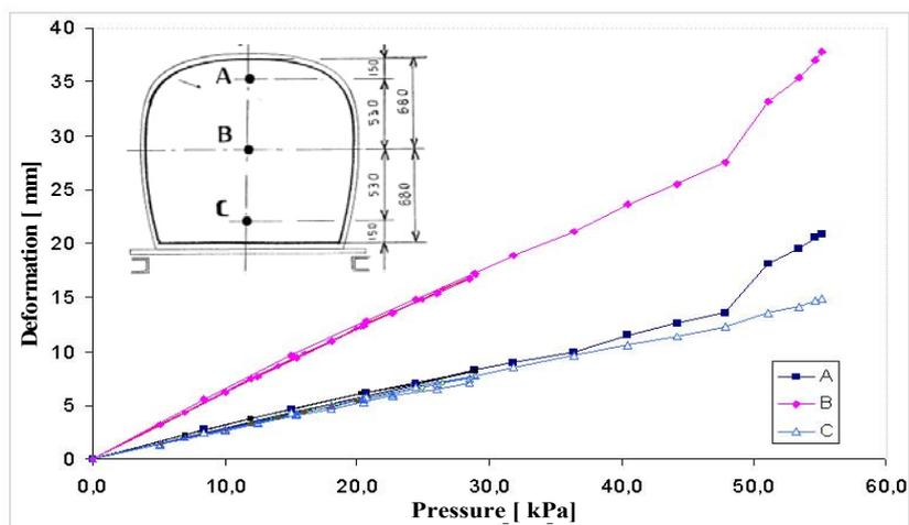
Figure 9: Deformation vs. pressure diagram during the residual static test
