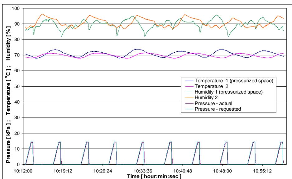
Figure 5: Typical curves of measured values (temperature, humidity and pressure) during the test
