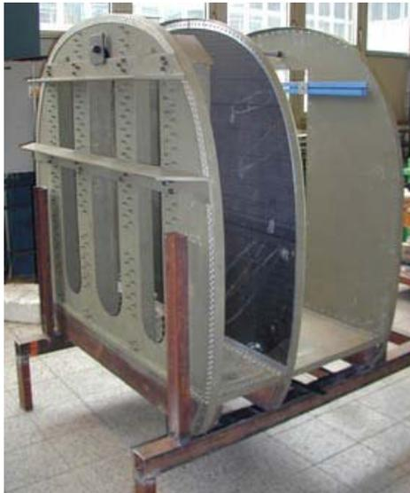
Figure 3: Location of the bulkhead inside of the testing box
