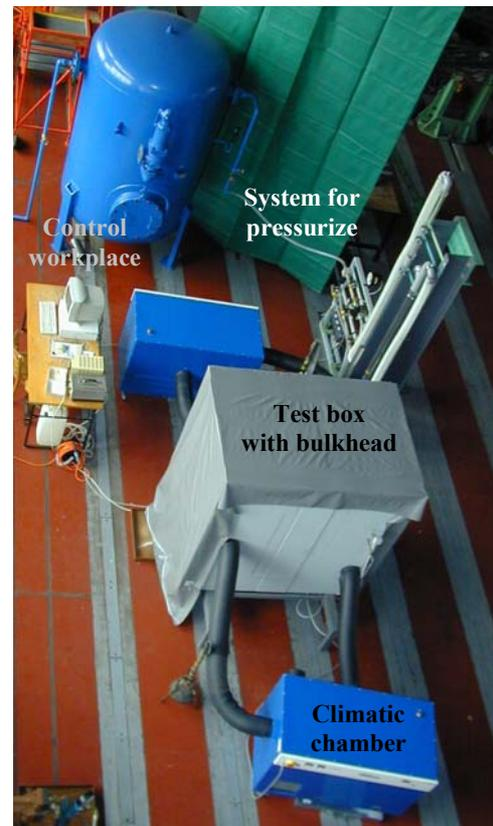
Figure 4: Configuration of the composite bulkhead test
