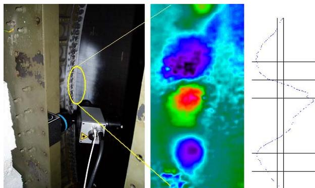
Figure 6: Detail of one full-field measurement (format A4) by shearography system Q-800
