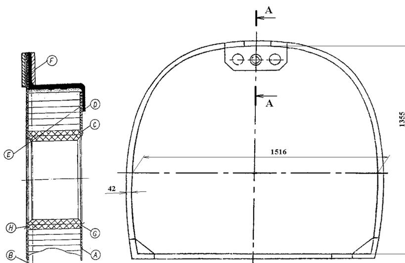
Figure 1: Schematic outline of the pressurized bulkhead structure configuration
