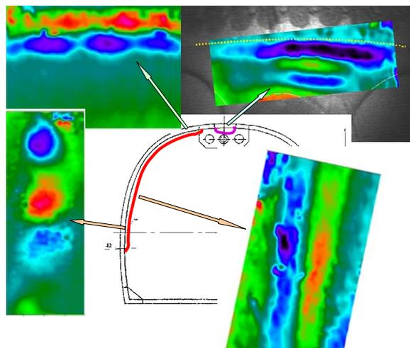
Figure 7: Results from nondestructive shearography inspection whole pressurized side of the bulkhead
