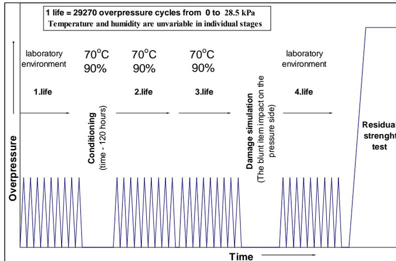
Figure 2: Loading programme for the bulkhead test with environmental simulation
