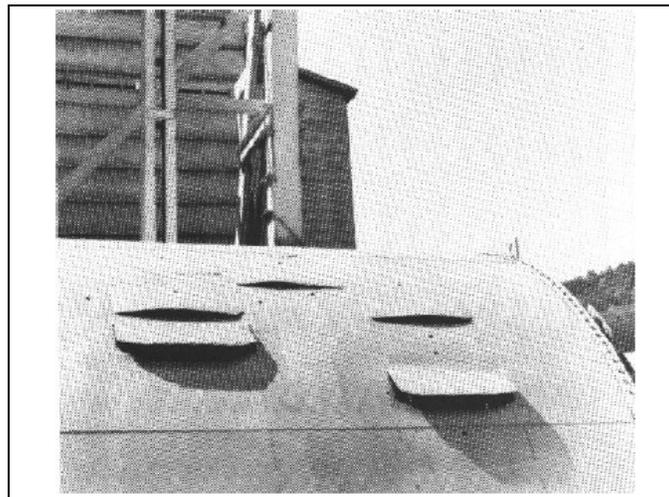
Figure 1: Crack turning and flapping in Boeing 707 test panel [1]
