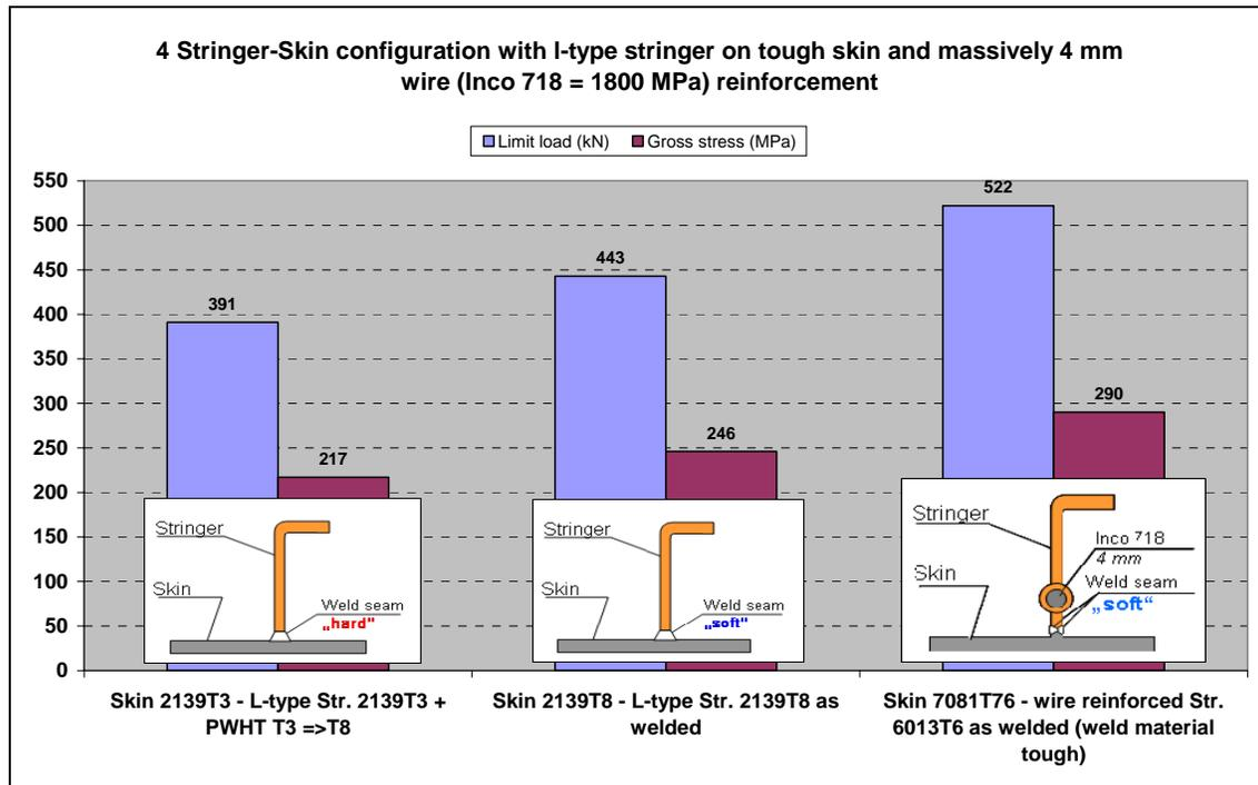
Figure 15: 4-Stringer test panels with laser beam welded stringer
