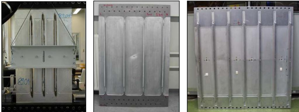
Figure 9a - c: Panel configurations with pre cracked middle stringer (for 3 or 7 stringer panels) or center crack (4 stringer panels)
