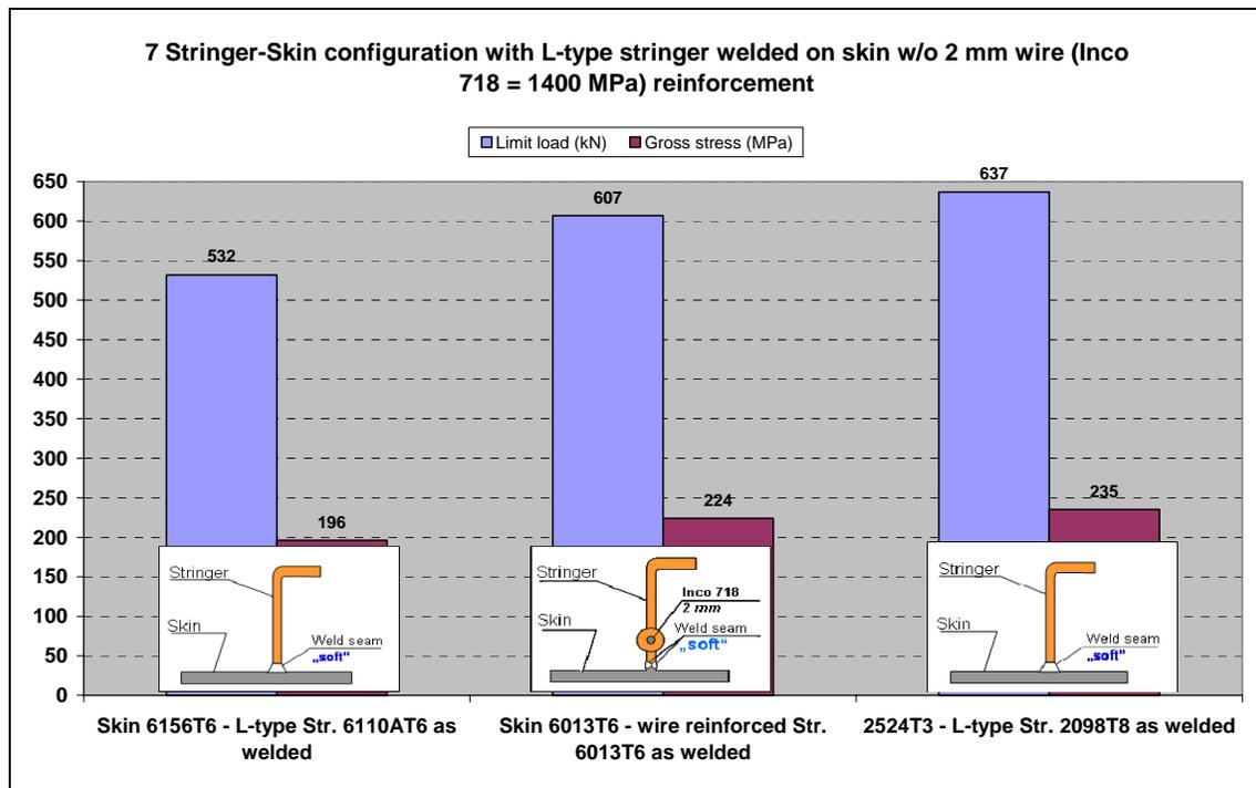
Figure 14: 7-Stringer test panels with laser beam welded stringer
