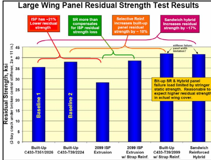
Figure 4: Comparison of residual strength in integral and built up 5 stringer test panels [7]
