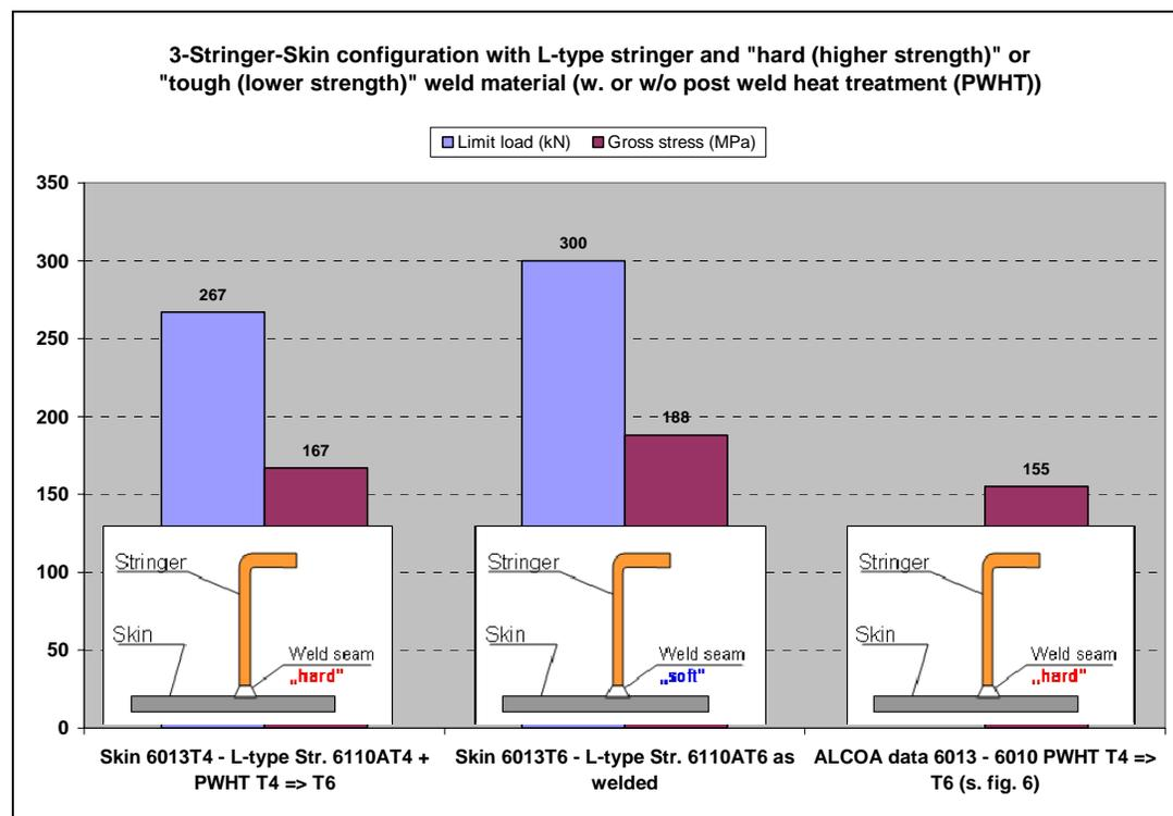
Figure 11: 3-Stringer test panels with laser beam welded stringer
