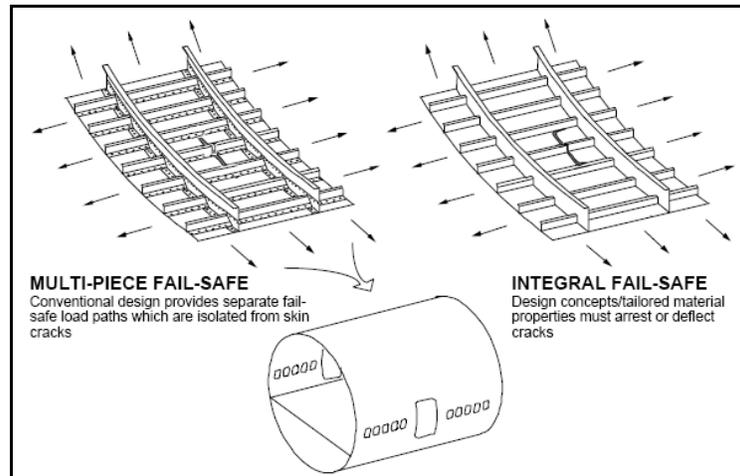
Figure 7: Fail safe in built up and integral structures [1]
