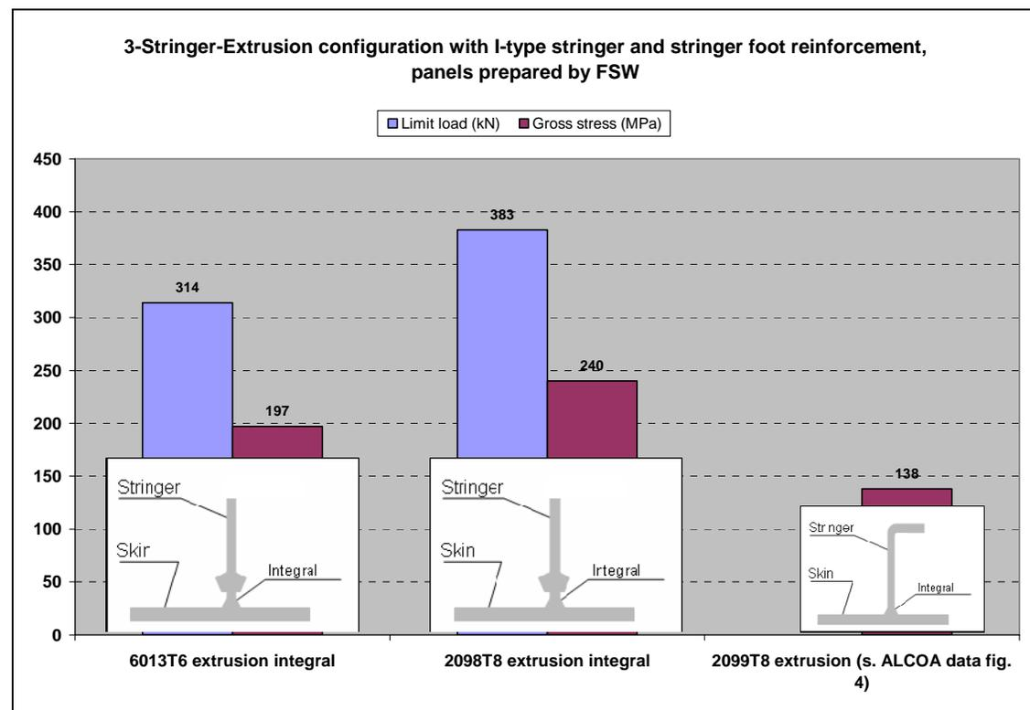
Figure 12: 3-Stringer test panels made from extrusions by Friction Stir Welding
