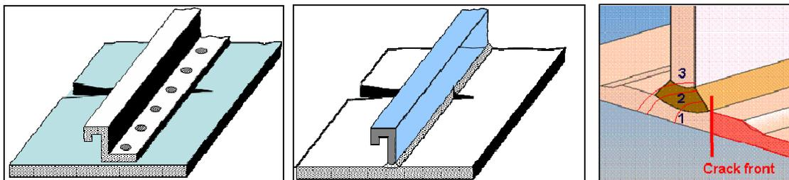
Figure 8 a-c: Differences in crack bridging in riveted and welded T-joint configurations [8] [10]
