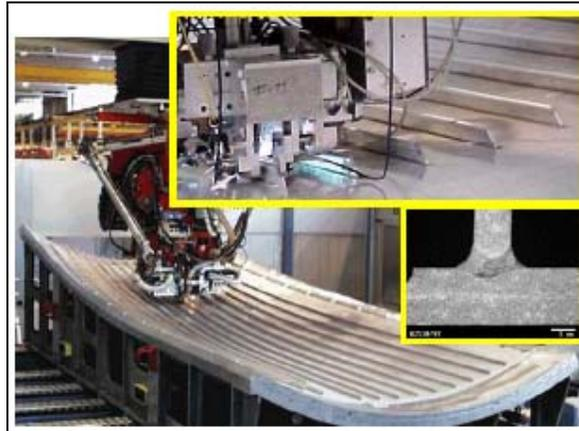
Figure 5: Laser beam welding of stringer to skin in spherical shaped shells for Airbus A318 [3]
