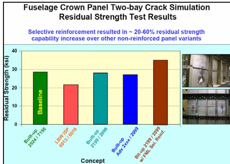
Figure 6: Comparison of residual strength in integral (laser welded) and built up 5 stringer test panels [9]
