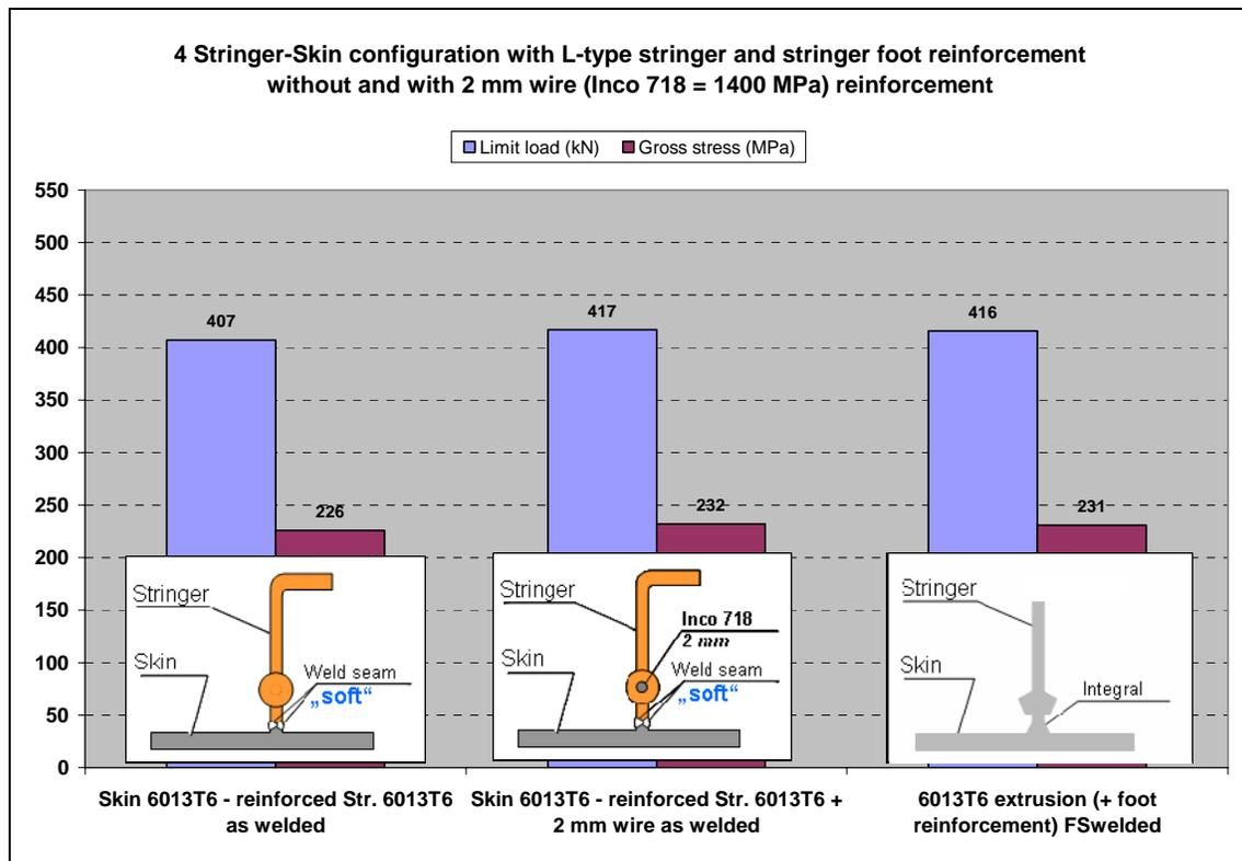
Figure 13: 4-Stringer test panels with laser beam welded stringer compared to a test panel made from extrusions
